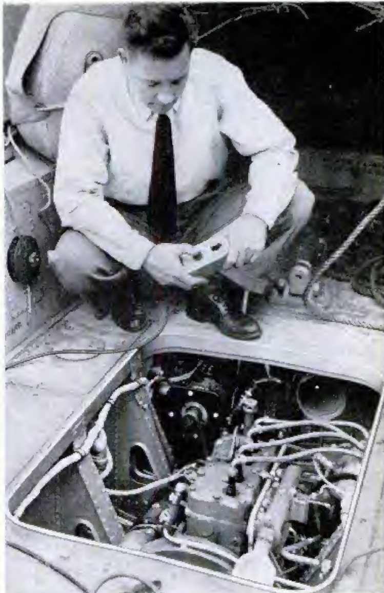
Above, engine is mounted below deck of the craft and can be entirely controlled by unit in hands of engineer. Or, if the passengers are too weak, the operation can be performed from plane by radio. Below, ladder drops into water for survivors
